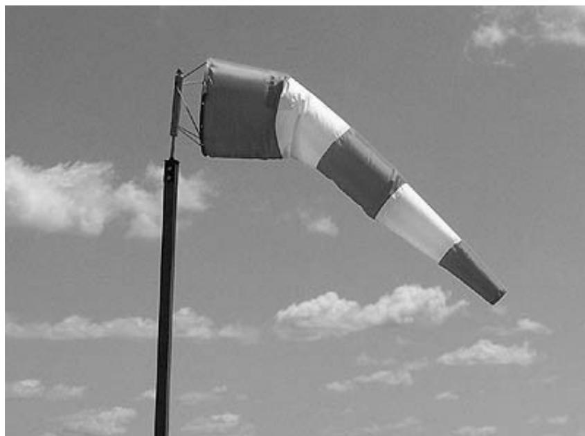
A **windsock** is a fabric tube designed to show the direction and speed of wind.
